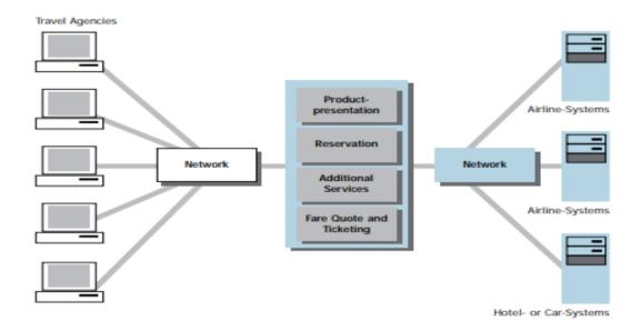
Fig. 3. Principal Structure of Global Distribution System. Source: (Authors)
