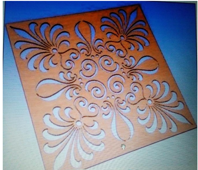
Figure 2-1: Example of wood carving by 2-axis CNC router.
