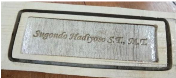
Figure 4-18: Marking results on wood board.
