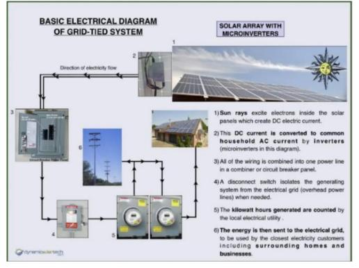
Plate 3.1 Basic Electrical Diagram
