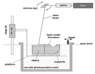
Figure 4: Sketch of the stereo lithography process.
