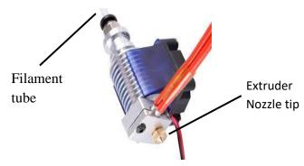
Figure 6: The exploded view of the Extruder Nozzle and a filament
