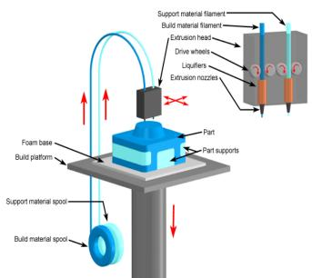
Figure 7: Schematic Representation of FDM Process
