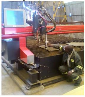
Figure 33: CNC Profile Cutter – Mufulira Mopani Copper Mine workshop.
