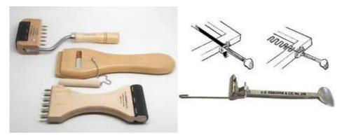
Figure 7: Webbing Stretchers and Webbing Puller Stretcher
