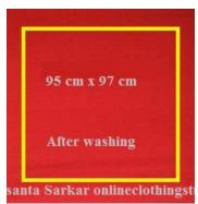
Lay the specimen on a flat table and remove creases but don't stretch the fabric. Measure the fabric length and width following marking points and note it.
