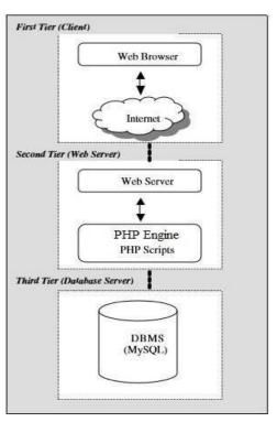
Figure 1. The three-tier architecture model of web database
