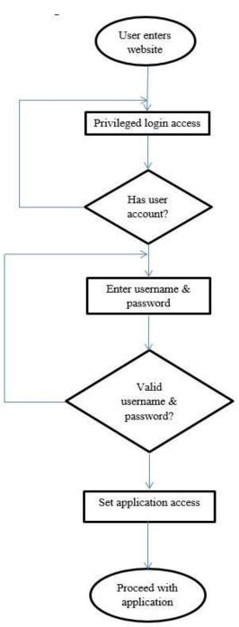
Fig. 33 - Website data flow diagram
