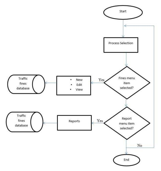
Fig. 34 - System process flow diagram
