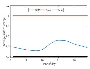
Fig. 6: Charging and discharging states of storage system
