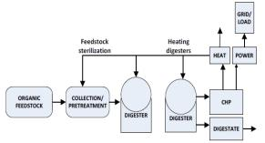
Fig. 2: Schematic of the biogas system
