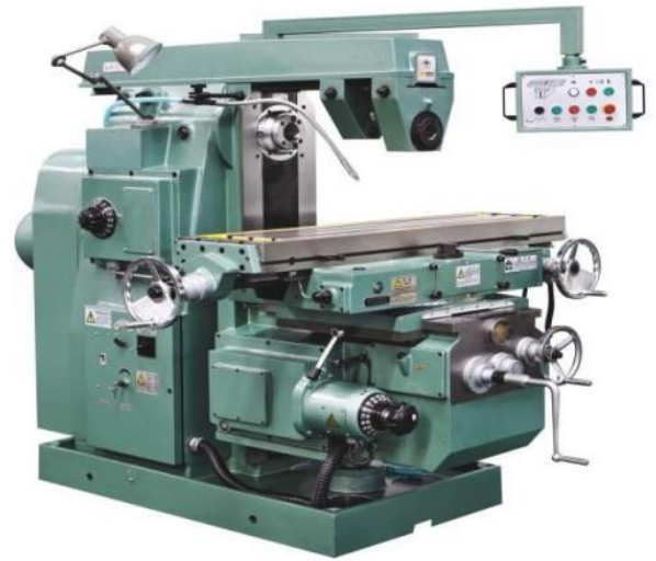
Figure 2. 3: Knee type 3-axis CNC machine Source: (Anon., 2016)
