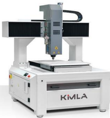
Figure 2. 5: Bed type 3-axis CNC machine
