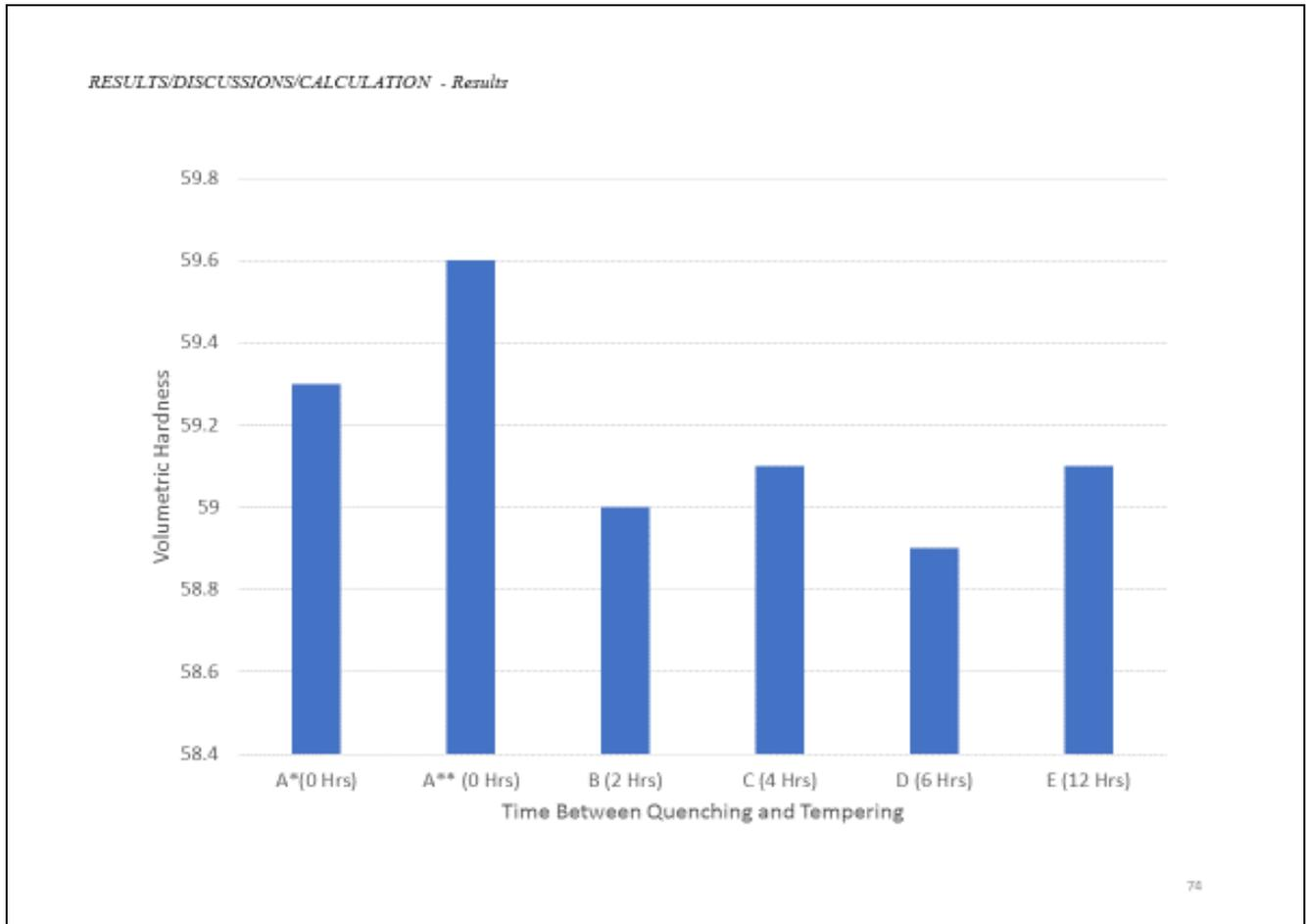
Figure 11: Graph Showing Volumetric Hardness of the samples (SOURCE: Author)
