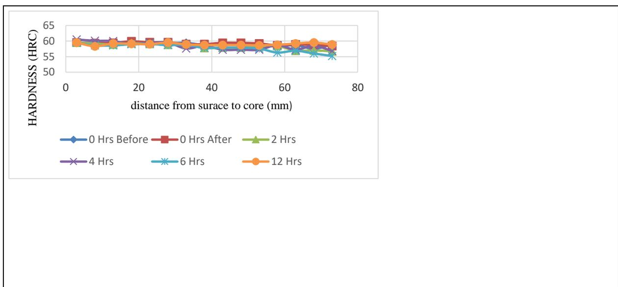
Figure 10: Graph Showing the hardness profile (SOURCE: Author). Figure 10 shows the hardness profile obtained from 0Hrs (Before and After), 2Hrs, 4 Hrs., 6Hrs and 12 Hrs. holding time before quenching.
