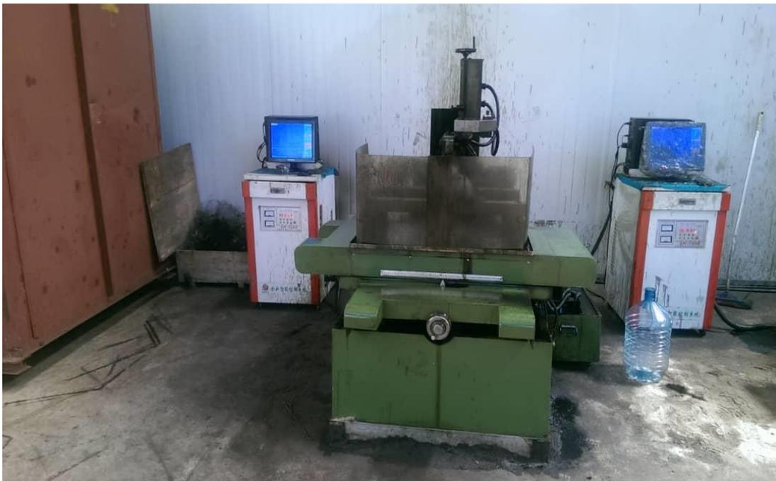
Fig. 3: Picture of an EDM Cutting Machine. (SOURCE: Author)
