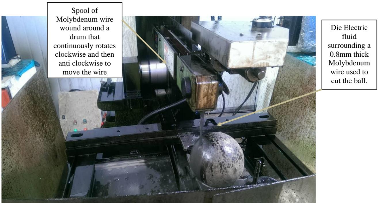
Fig. 5: Picture of a Mill Ball Sample Being Cut on an EDM Cutting Machine (SOURCE: Author)
