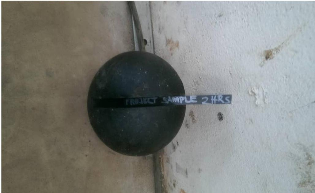
Fig. 6: Picture of an EDM Cut Sample in the cut Slot (SOURCE: Author)
