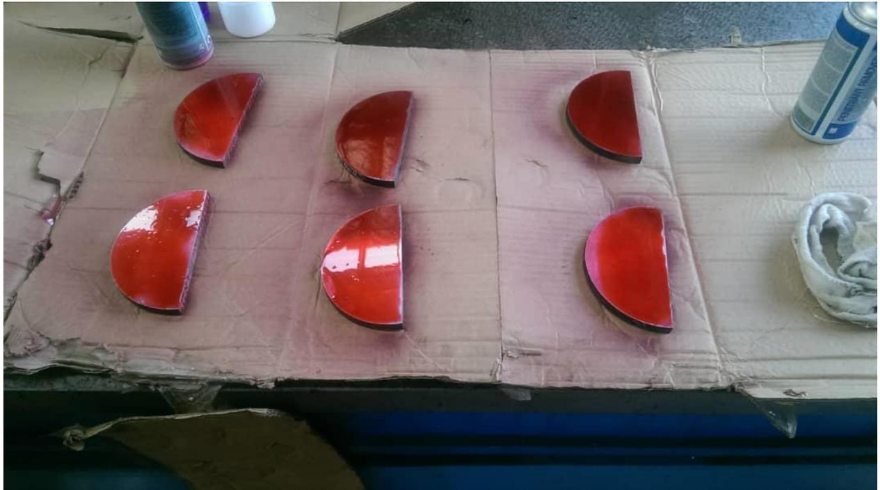
Fig. 13: Cut and Polished Sample undergoing NDT- Liquid Penetrant Tests (SOURCE: Author)
