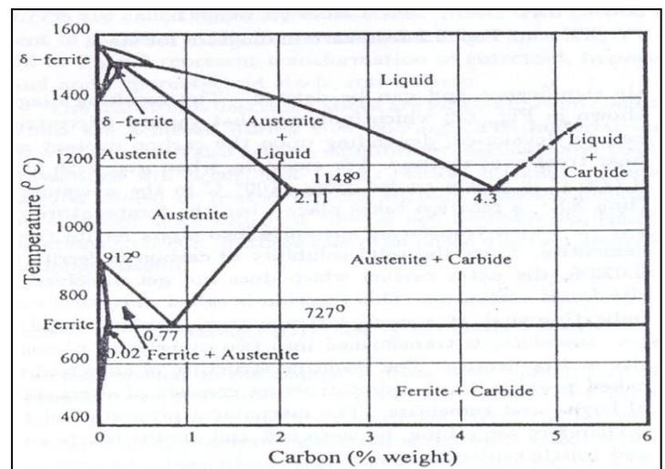
Fig. 1: Iron-Carbon Phase Diagram (Source: <http://panit.iid.ac.in/~pmpandey>)
