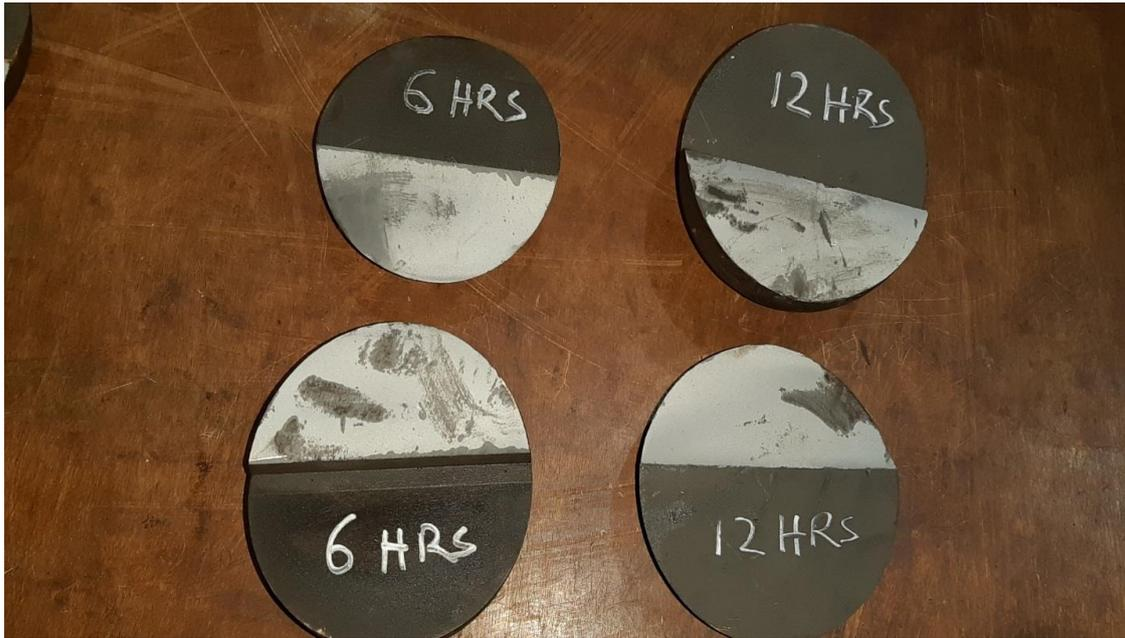
Fig. 12c: Internal of Split Balls (6 Hrs. and 12 Hrs.) (SOURCE: Author)
