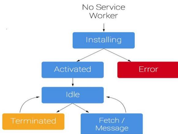
Figure 11 illustrates a simplified version of a service worker lifecycle on its first installation.
