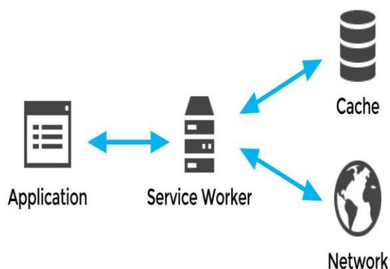
Figure 3 UML activity diagram for the workflow of an offline capable app implemented by service workers (Shepherd, Eric, Mills, Chris and Sabiwara. 2016 )
