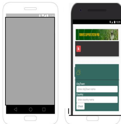
Figure 4 Illustration of a PWA's application shell without content (left) and filled with content (right)
