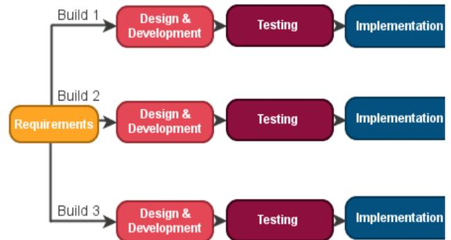
Fig. 7. Iterative Software Development Process
