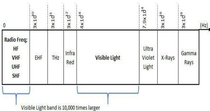
**Figure 1 - Radio Frequency vs. Visible Light Frequency Bands. Courtesy of author.**
