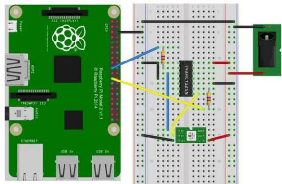
**Figure 7 - TX Module Layout Diagram.**
