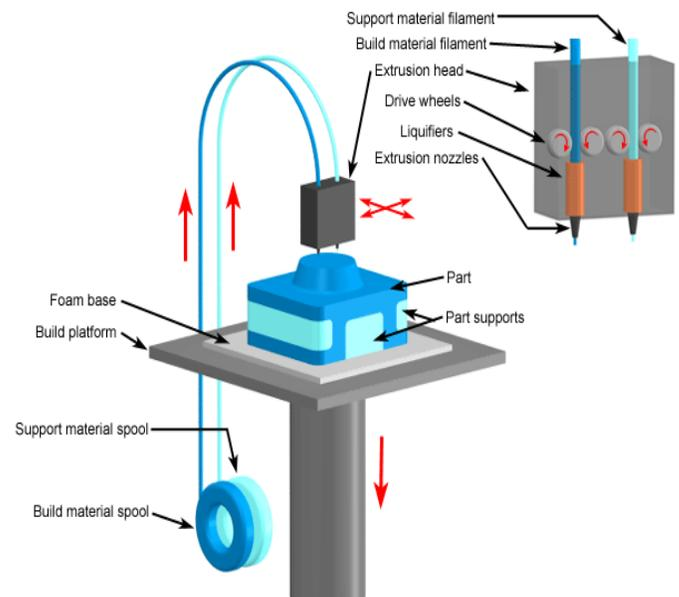
Figure 7: Schematic Representation of FDM Process
