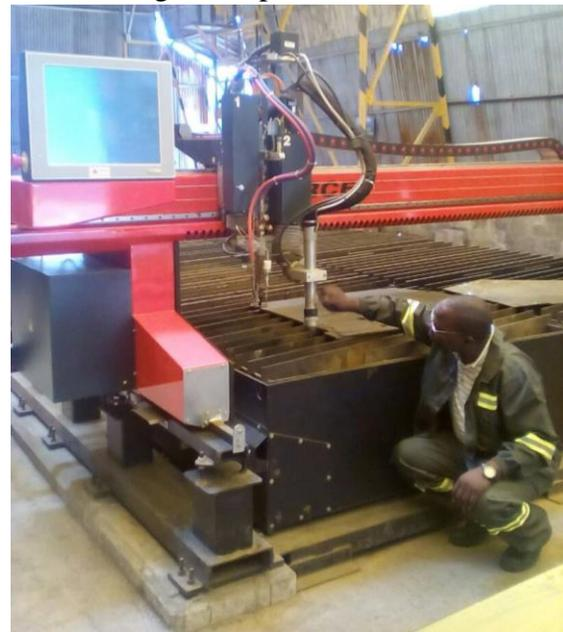
Figure 33: CNC Profile Cutter – Mufulira Mopani Copper Mine workshop.
