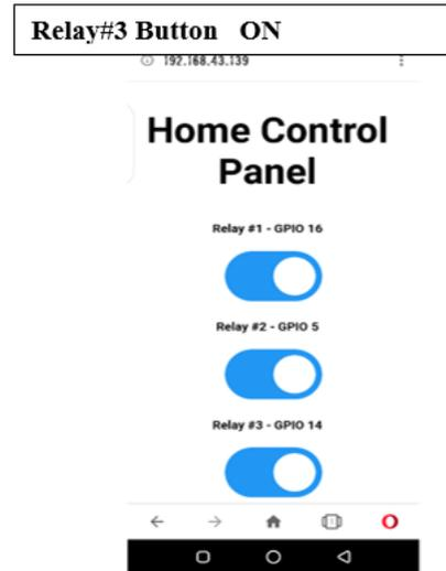
**Relay#3 Button or Blynk #3 Button Corresponding bulb ON**
