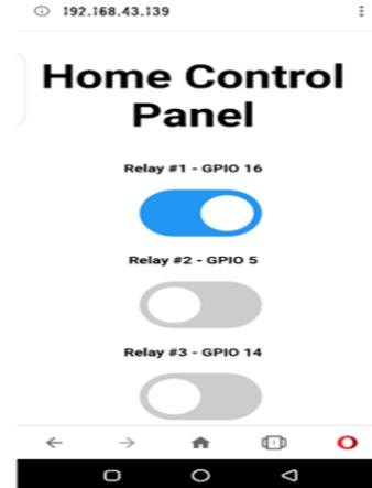
**Relay#1button or Blynk #1button Corresponding bulb ON**
