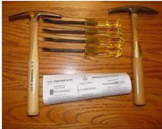
Figure 9: Staple lifter hammer
