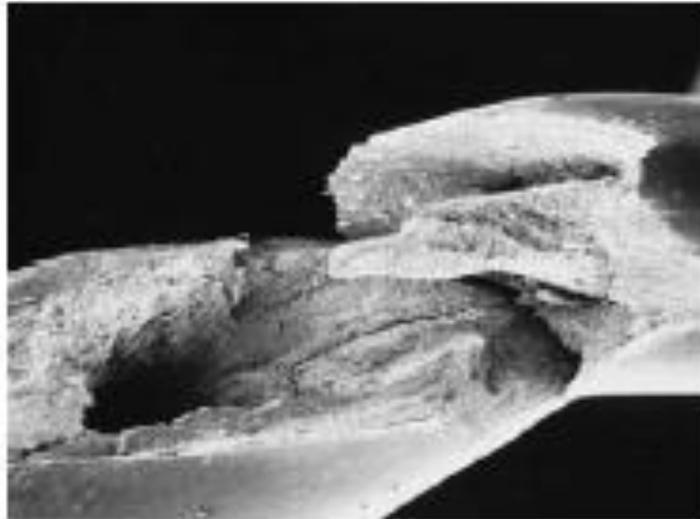
Figure 6 Wire Break due to Centre Burst Source: (Wright, 2011)
