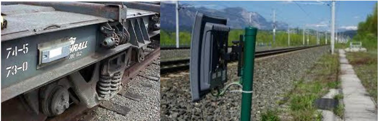
Figure 2. Above shows the passive tag on a rail car and the wayside reader
