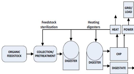
Fig. 2: Schematic of the biogas system
