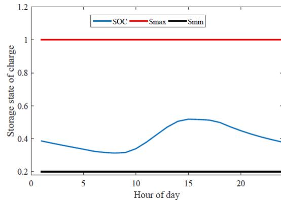
Fig. 6: Charging and discharging states of storage system
