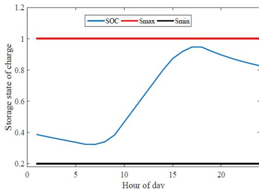
Fig. 4: Charging and discharging states of storage system
