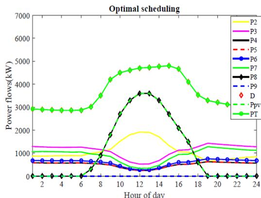
Fig. 5: Optimal dispatching with reduced PV output
