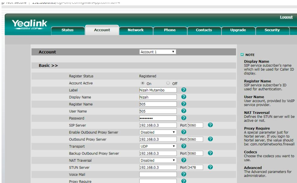
Figure 1.3: VoIP configuration in the client side (IP Phone)
