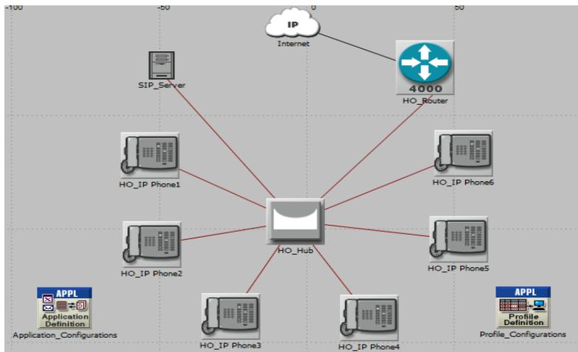
Figure 4.1.4: Scenario 1 VoIP LAN topology with 6 Nodes
