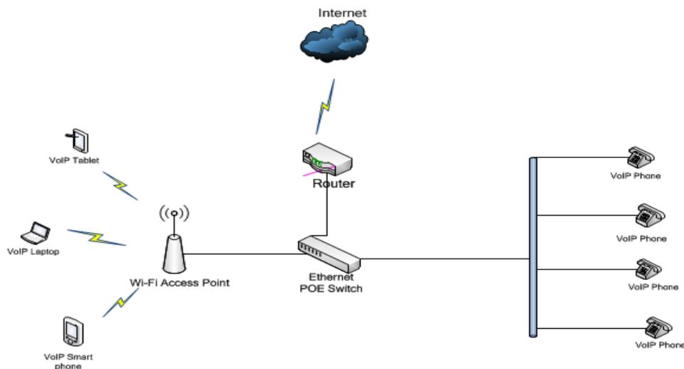
Figure 1.1 VoIP on Ethernet cable and wireless
