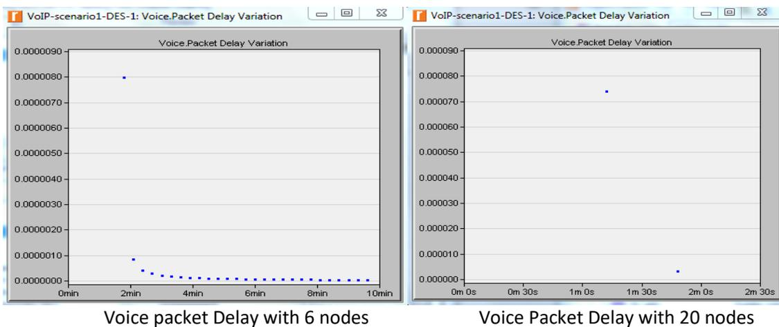
Figure 5.1.2: Simulation results for voice packet delay.
