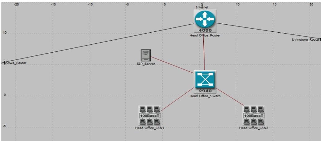
Figure 4.1.9: VoIP LAN Setup at Head Office – Lusaka
