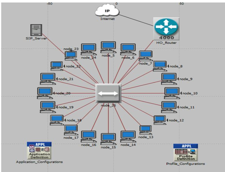
Figure 4.1.5: VoIP LAN Network with 20 stations using a Hub
