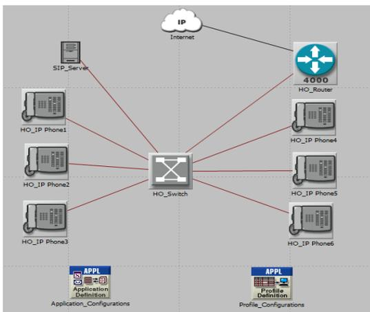
Figure 4.1.6: VoIP LAN using a switch with 6 Nodes
