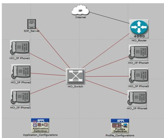
Figure 4.1.6: VoIP LAN using a switch with 6 Nodes
