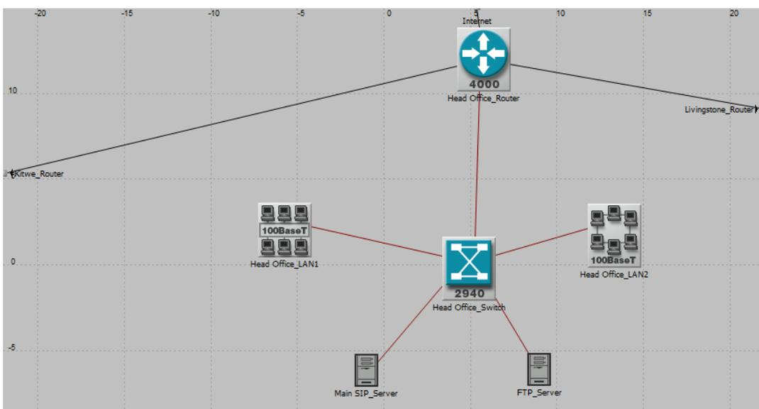
Figure 4.1.12: VoIP WAN setup with FTP services running
