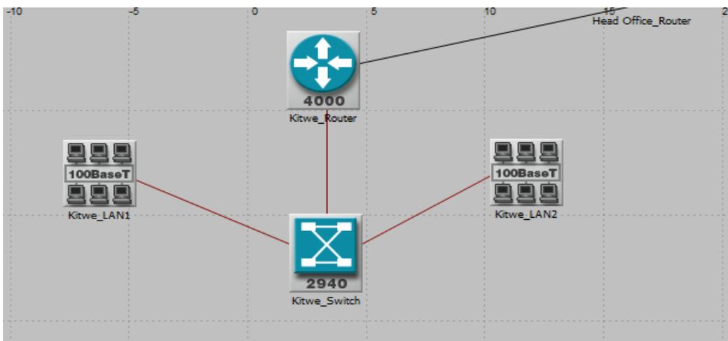
Figure 4.1.10: VoIP LAN setup in the Northern Region – Kitwe
