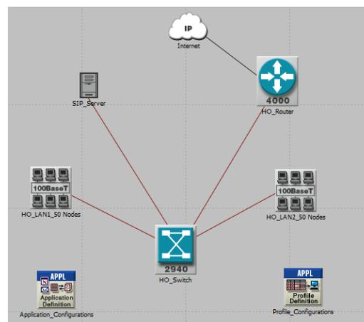
Figure 4.1.7: VoIP LAN setup using the switch with 100 Nodes
