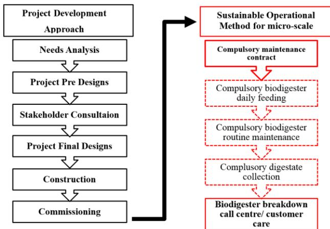
Fig. 4: Proposed sustainable biodigester operational method
